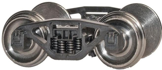
Many freight cars built in the 1920s were equipped with Dalman trucks. The Dalman 2-level truck design used additional springs to give a smoother ride. Railroads using this version include Chesapeake and Ohio, Chicago Great Western, Illinois Terminal, L&N, Milwaukee Road, M-K-T, Nashville Chattanooga and St. Louis, Pere Marquette, and many Texaco 10,000 gallon tank cars.
