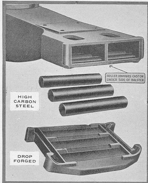
Fig. 2211—Barber Lateral Motion Device Dismantled
